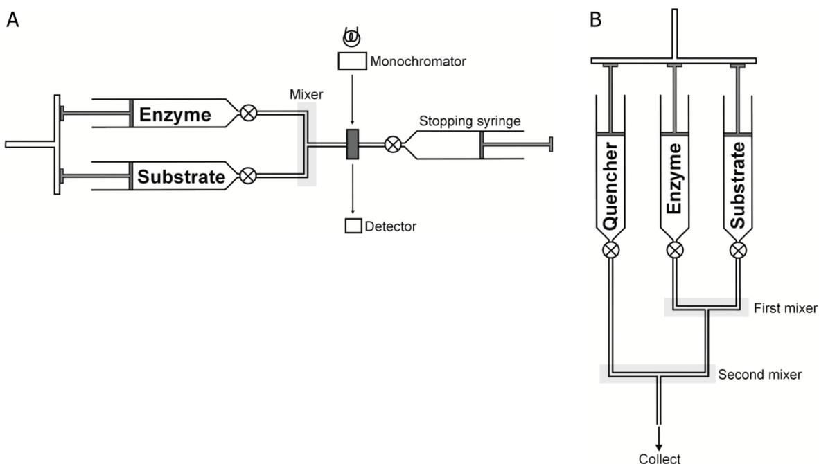
**Figure 6.** Schematic diagrams of stopped-flow (A) and quenched-flow (B) apparatus.
